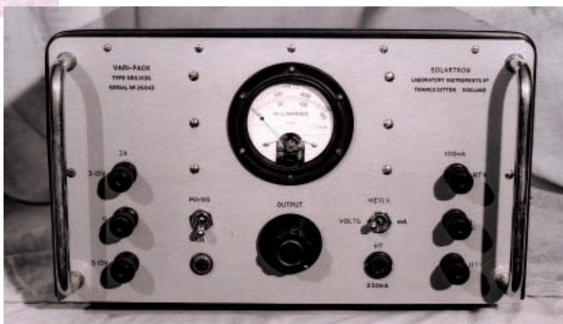
● Fig. 6: The valve regulated high tension power supply, now fully working. Before being nurtured back to good health it was heading for the rubbish skip (see text).
