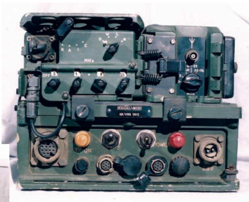
● Fig. 3: The PRC-351 transceiver with amplifier (right) and vehicle interface below (see text).
