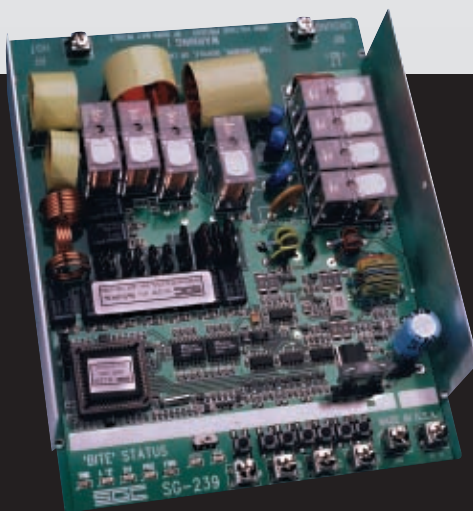
● There are a variety of a.a.t.us. available for Amateur Radio use. This version, the SG-239 can be mounted inside a building or a vehicle.
