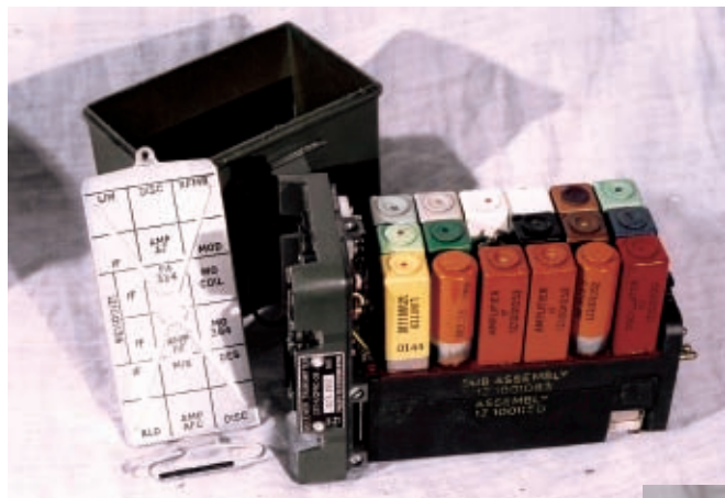
● Fig. 5: The internal modular construction inside the CPRC-26 radio.
