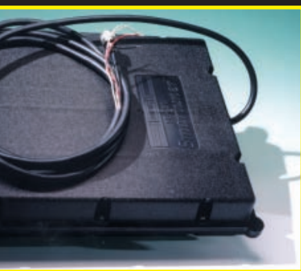
● In use the SGC automatic antenna tuners (a.a.t.us) only require r.f. drive and a 13.8V power supply).
